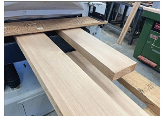
The wood is milled to 1 3/4" for the door stiles and rails
