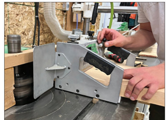
The shaper cuts for the cope and stick joinery
